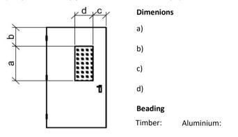
Note: sizes shown refer to Clear View. For Fire Doors, minimum b) dimension must be 200mm and minimum c) dimension must be 150mm. Fire Doors rated FRR-/90/-sm and above can only have VP a) dimension 600mm and b) dimension 100mm with Steel beading
